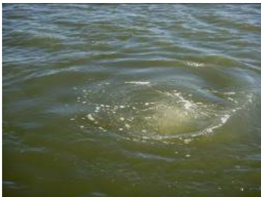
Actual diameter of bubble disturbance area is about 4 feet at each aerator
