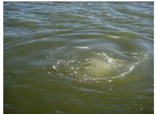
Actual diameter of bubble disturbance area is about 4 feet at each aerator
